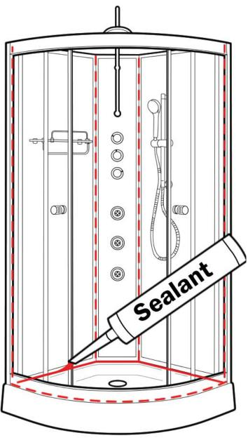
DO NOT PUT SEALANT INTO THE WATER RETURN CHANNELS
